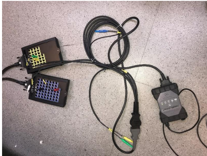
Image 1: Measurement Cable OBD-Plug
